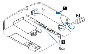
At the same time two tabs on the inside of the cable cover will be engaged in the responding grooves of the projector.
