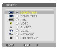
2. Press the SELECT ▼ or ▲ button to select [NETWORK] and press the ENTER button. The [NETWORK] menu will be displayed.
