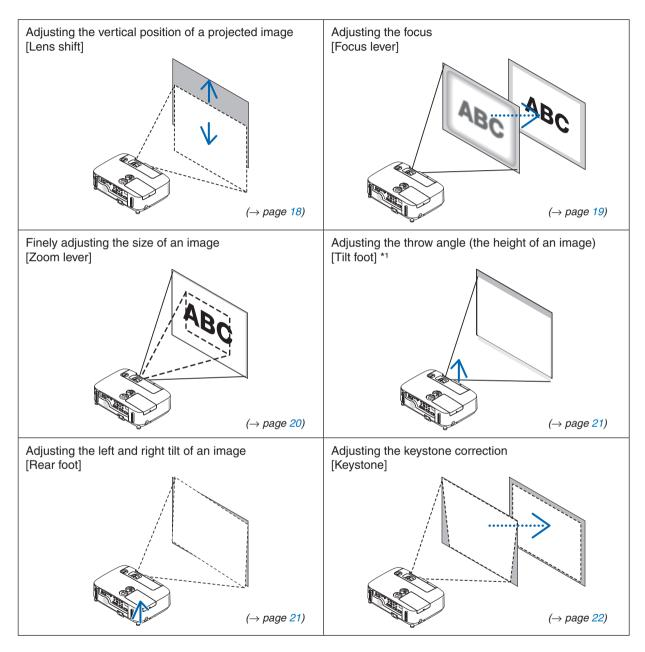
NOTE\*1: Adjust the throw angle (the height of an image) when the image position is higher than the lens shift adjustable range.
