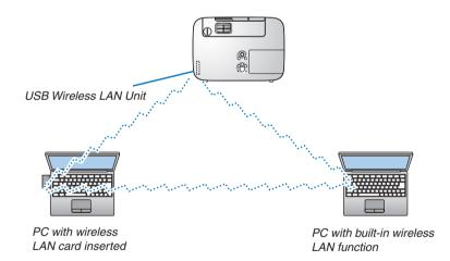
To enable direct communication (i.e., peer-to-peer) between computers and projectors, you need to select the Ad Hoc mode.
