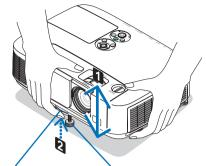
Adjustable Tilt Foot Lever Adjustable Tilt Foot
