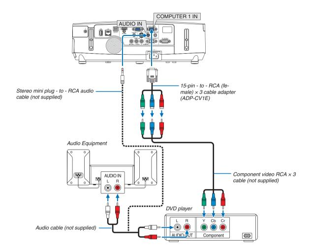
A component signal will be automatically displayed. If not, from the menu, select [SETUP]  $\rightarrow$  [OPTIONS(1)]  $\rightarrow$  [SIGNAL SELECT]  $\rightarrow$  [COMPUTER1] or [COMPUTER2], and then place a check mark in the Component radio button.
