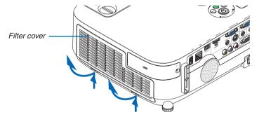
2. Remove the filter unit by pulling out the tab.
