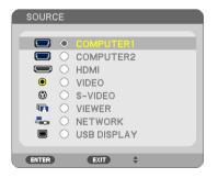
2. Press the SELECT ▼ or ▲ button to select [NETWORK] and press the ENTER button. In the screen, the [APPLICATION MENU] menu is displayed.
