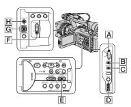
You can adjust the brightness of a picture with the EXPOSURE/IRIS dial G. You can assign any one of [EXPOSURE1] (the default setting), [EXPOSURE2], [IRIS] and [AE SHIFT] to the EXPOSURE/IRIS dial G from the menu (p. 69).
