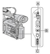
You can adjust the white balance according to the light of the recording environment. You can set two sets of white balance adjustment data separately in memory A and memory B for two different recording conditions with A and B. During recording, you can select the setup data with the SEL/PUSH EXEC dial. The setup data will be retained as long as it is not readjusted even if the power is disconnected.
