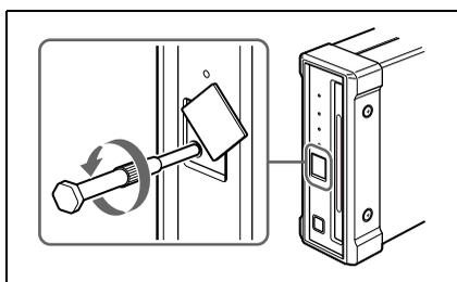
After ejecting the disc, it is not necessary to return the screw to its original position. The next time the unit is powered on, normal operation will resume.
