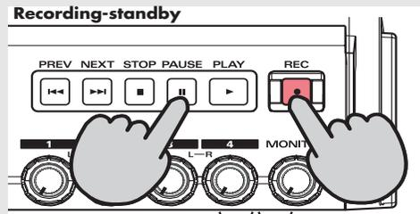
The R-4 Pro enters recording standby mode. During recording standby, the **[REC] button** blinks and the display alternates between **REC** and **STANDBY**.
