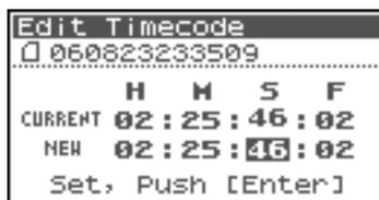
\* *H:M:S:F: indicates Hours:Minutes:Seconds:Frames, respectively. The F value differs according to the Frame Rate value in the timecode Setup.*
