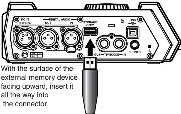
With the surface of the external memory device facing upward, insert it all the way into the connector
