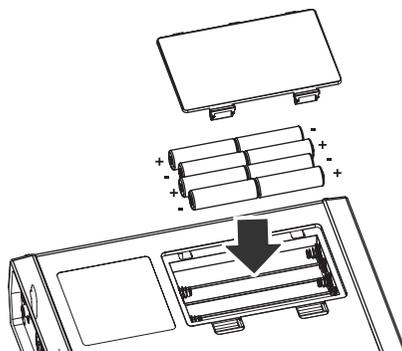
**3** Insert eight AA batteries into the battery compartment, making sure to observe the correct polarity (+ and - symbols).
