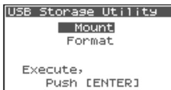
When the connection to an external memory device is mounted, the USB Storage Utility starts as shown in the figure to the right.
