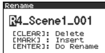
Use the **[CLEAR]** button to delete a character and the **[Mark]** button to insert a character. Use these buttons to edit the name as desired.
