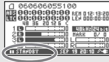
When recording is paused, the **[REC] button** blinks. In addition, the display alternates between REC and PAUSE.
