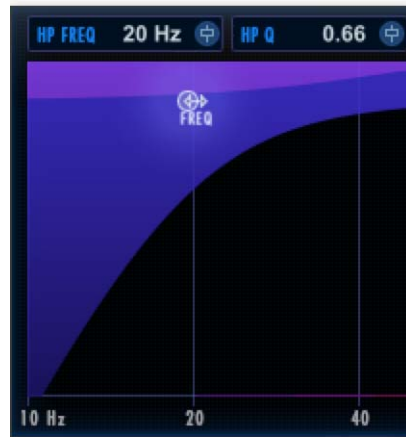
Adjusting the Frequency setting on the Frequency Graph
