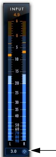
Input section with Meters and Input Level control
