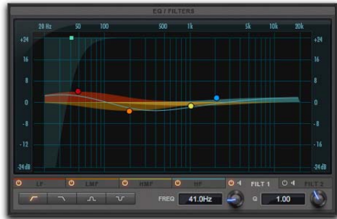
EQ/Filters section, Filter 1 tab shown
