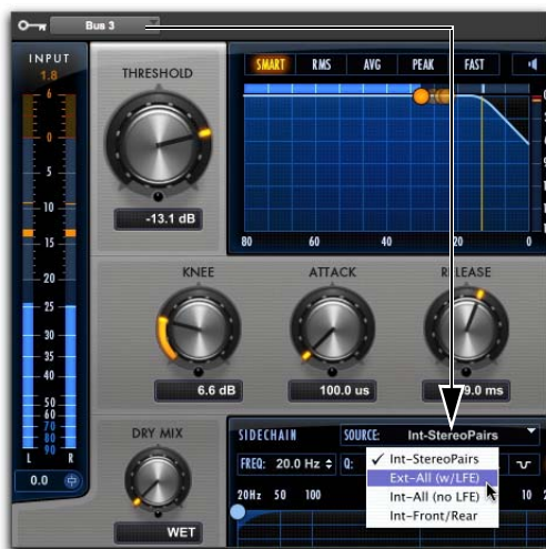
Selecting the Source for side-chain processing
