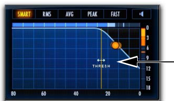
Cursor indicates Threshold adjustment
