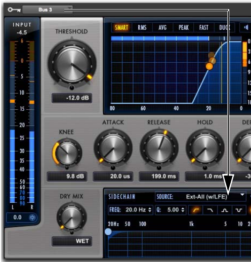
Configuring a key input for side-chain processing
