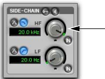
HF frequency controls
