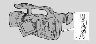
The zebra pattern is a series of diagonal stripes that appear in the viewfinder to highlight areas of overexposure. Use it as a guide to set the aperture (iris) and shutter speed.
