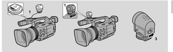
Using the optional Video Light enables you to record even in dark rooms. This VL-3 Video Light attaches to the camcorder's *s* advanced accessory shoe for cable-free operation and is powered by the camcorder's power supply.
