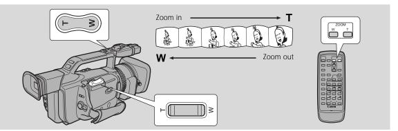
This camcorder is equipped with 20x optical zoom and 100x digital zoom. Optical zoom and digital zoom can be operated from either the side grip, the camcorder handle or the wireless controller.
