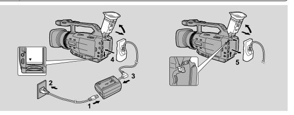
Use the power adapter and the DC coupler to provide your camcorder with instant power from an household power socket.
