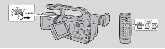
When you play back a tape that was recorded in 12-bit mode, you can set the audio output to stereo 1 (the original sound), stereo 2 (any new sound, dubbed to the tape after recording), or mix the balance between the two.
