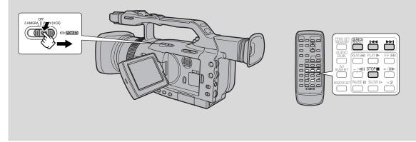
This allows you to move quickly through still images (photo search), between different days or areas of recording (date search), or index signals ( $\square 57$ ) recorded anywhere on a tape (index search).
