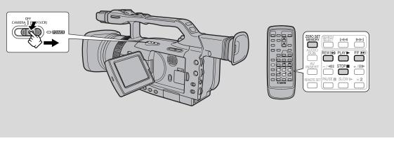
Use the wireless controller to mark a point on a tape to which you wish to return following the playback.
