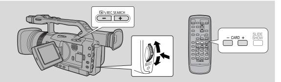
This section describes how to protect the still image from the Card Operation submenu when displaying an index screen in CARD PLAY (VCR) mode (including the way to cancel the setting). You can also protect a still image through the File Operation menu ( $\square$  121).
