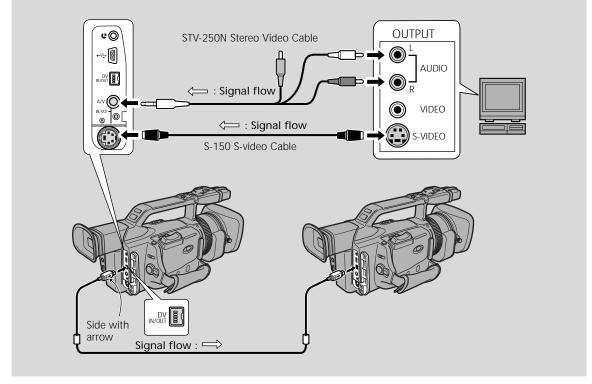
Above illustration shows the connection using a S-video cable. You can also connect the yellow plug to the VIDEO terminal instead.
