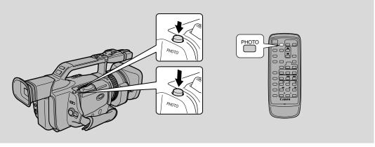
You can record still images like photographs. The camcorder records the picture and sound to tape for several seconds. The exposure is automatically adjusted.
