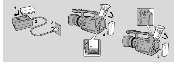
Your battery pack was partially charged before it left the factory. It should have enough power for you to check that your camcorder is working properly. However, you must charge the battery pack fully if you want it to power the camcorder for more than a few minutes.
