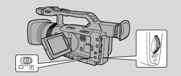
The camcorder provides you with a choice of seven recording programs. They use different combinations of camcorder settings in order to adjust the exposure and other functions to match the recording situation.
