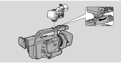
The MA-300 Microphone Adapter enables you to input audio to the camcorder with XLR connector equipped microphones, and to convert video signals for the BNC connector. Refer to the MA-300 Microphone Adapter instructions for further details.
