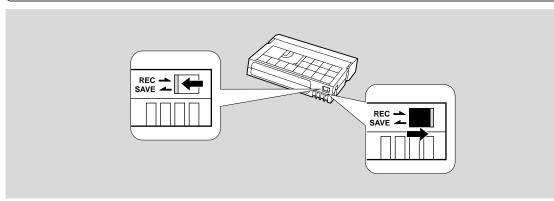
To protect your recording from accidental erasure, slide the tab on the cassette so that it exposes the hole. (This switch position is usually labelled SAVE or ERASE OFF.)
