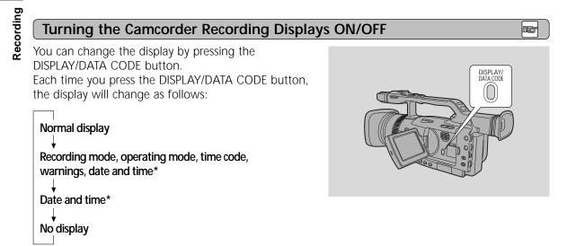
\* Appears when GUIDE INFO is set to D/T DISPLAY in the DISP. SET UP submenu (CAMERA menu).
