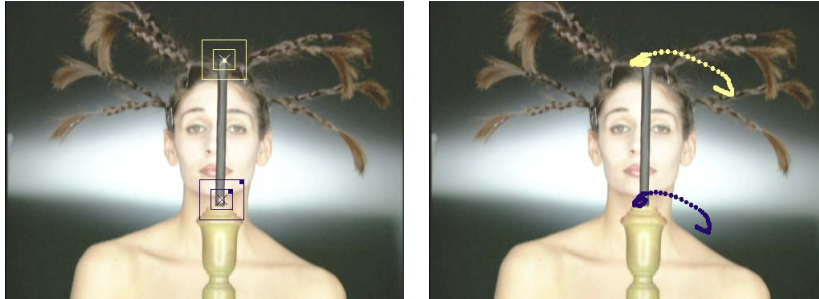
The tracking boxes located over the targets (left), and the generated tracking data points for the entire clip (right).
