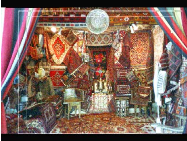
Field of view display for Avid Pan & Zoom effect: field of view rectangle (outer rectangle), Safe Action area (inner rectangle), and crosshair (center)
