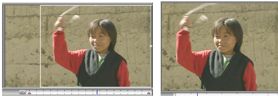
Pan and Scan example: original media with the Pan and Scan wireframe in 16:9 mode (left), and results of the Pan and Scan effect in 4:3 mode (right)
