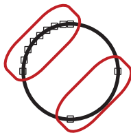
Unnecessary number of control points (left) and minimum number of control points (right) for describing the curve
