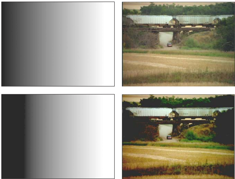
Example of a Levels adjustment that changes the Input Black Point value to 60 (all other values are defaults): unadjusted images (top) and adjusted images (bottom)
