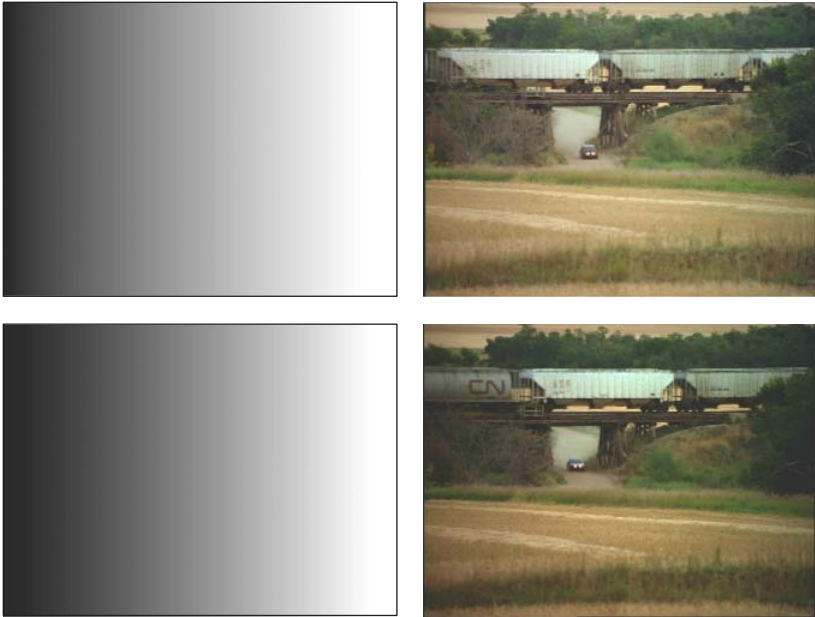
Example of a Levels adjustment that changes the Output Gray Point value to 100 (all other values are defaults): unadjusted images (top) and adjusted images (bottom)
