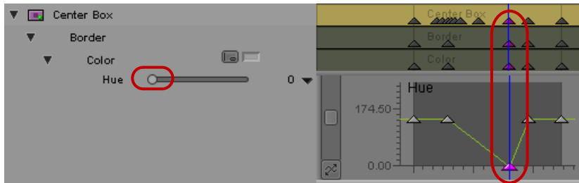
Active parameter (left) and keyframes added when you use the Add to Active Parameter command (right)
