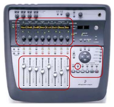
Layout of the 002. Top: Console/channel view section (contains a pan knob for each track). Bottom left: Fader section. Bottom right: Transport and Navigational controls section (the Mix button is highlighted within this section).
