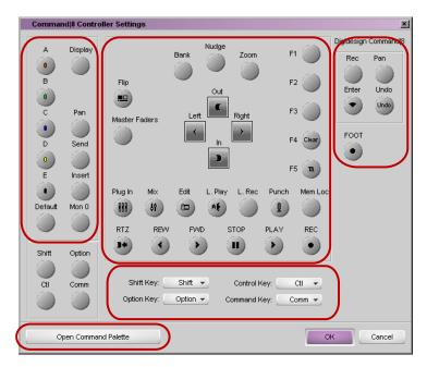
Groups of controls in the Command 8 Controller Settings dialog box. Top, left to right: Console View controls, Transport and Navigation controls, Display Controls and Foot Switch. Center: Keyboard Modifier switches. Bottom: Open Command Palette button.
