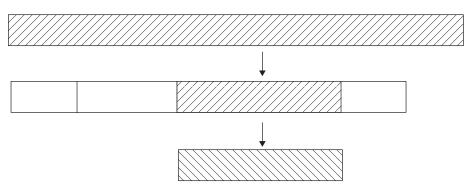
Top to bottom: original DV25 clip, portion of DV25 clip edited into a sequence, and new clip created in 15:1s by consolidating and transcoding the sequence. Only part of the original clip is available in 15:1s.
