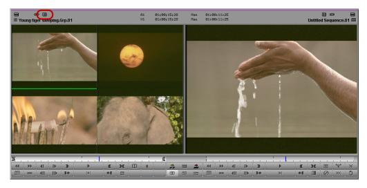
Quad Split Source view, with the four camera angle views in the Source monitor and the sequence or linecut in the Record monitor. The location of the Group Menu icon is highlighted.
