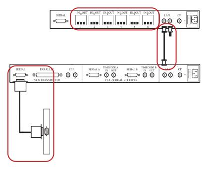
Top left: GPI terminals on the VLXi-GT GPI (for connections to external hardware). Top right: V-LAN connection (from VLXi-GT to V-LAN VLXi controller) and terminator (required when cable length is more than 50 feet (15.24 meters). Bottom: Serial connection from V-LAN VLXi controller serial port connector to serial port connector on your Avid system (or on a USB-to-serial adapter). Note that all cables are customer supplied.
