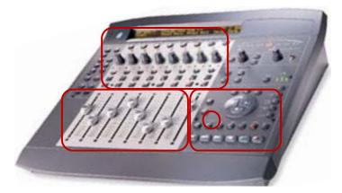
Layout of the Command|8. Top: Console/channel view section (contains a pan knob for each track). Bottom left: Fader section. Bottom right: Transport and Navigational controls section (the Mix button is highlighted within this section).
