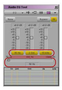
Example of shelf, parametric midrange, and turnover point information in the Audio EQ tool. The current value for all EQ parameters is 0 dB. Top: buttons that display turnover points (for the low shelf and high shelf curve) and bandwidth (in this case, 2 octaves) around the center point of the parametric curve. Bottom: EQ Range slider showing the center point of the parametric midrange curve.
