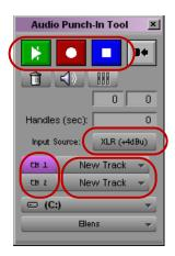
Audio Punch-In tool. Top, left to right: Play In/Out button, Record button, and Stop button. Center: Input Source menu. Bottom left: Input Channels buttons. Bottom right: Timeline Track menus.
