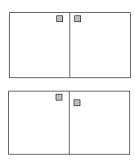
Example of color-framing boxes. Top: color sync signals are in phase and the boxes align horizontally. Bottom: color-sync signals are out of phase.
