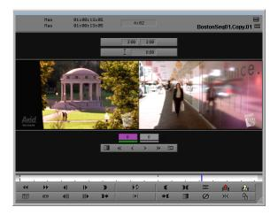
Quick Trim display — replaces Record monitor in single monitor view. Outgoing and incoming frames appear side-by-side on the right, with playback loop parameter controls above them, and with frame offset counters and Trim buttons beneath them.
