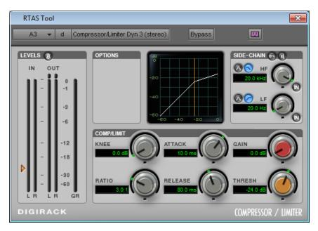
The Compressor/Limiter Dyn 3 plug-in window displayed in the RTAS too dialog box.
