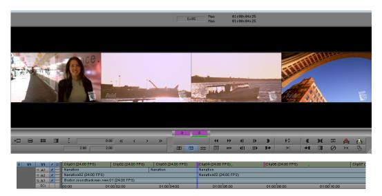
Four-frame display for slip and slide trimming. Left to right: outgoing video at position indicator, head and tail frames of the selected clip, incoming video at position indicator.
