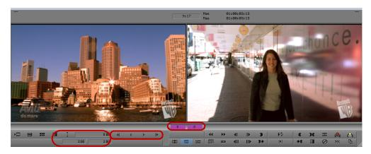
Big Trim display — replaces both monitors in two-monitor view. Outgoing frames appear on the left and incoming frames appear on the right. Bottom, left to right: Playback loop parameter controls, frame offset counters, and Trim buttons.
