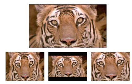
Example of downconversion formats. Top: the HD image. Bottom, left to right: Anamorphic, Letterbox, and Center Cut SD downconverted images.
