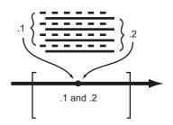
• Upper field is first: The upper field in the frame (odd-numbered lines, when the frame lines are numbered starting from 1) occurs temporally before the lower field, as shown in the following illustration. This arrangement is termed "upper field first" (or "lower field second").
