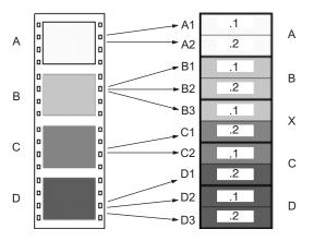
Relationship between four film frames (left) and five NTSC video frames (right). On the right, .1 indicates an odd field and .2 indicates an even field.
