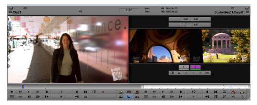
Small Trim display — replaces Record monitor in two-monitor view. Outgoing and incoming frames appear side-by-side on the right, with playback loop parameter controls above them, and with frame offset counters and Trim buttons beneath them.
