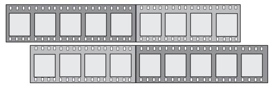
Example of zero-frame cutting with multiple strands. The handles are shown in lighter gray.
