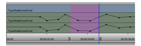
The following illustration shows the result after choosing Set Live Mix to Automation In/Out from the Audio Mixer Fast menu. The portion of the Timeline between the In and Out on Track A1 is changed to 0 dB and the same portion of Track A2 is changed by -45 dB to match the Live Mix settings. The system adds automation gain keyframes at the In and Out points and creates ramps from the In and Out points to the new value.
