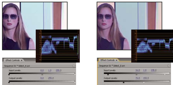
Original image (left); blacks and whites corrected to broadcast limits (right)
