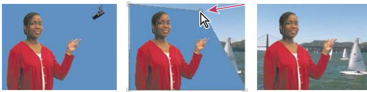
The microphone (left) is masked out by repositioning image handles in the Preview view of the Program Monitor (center), creating a garbage matte that is then keyed and superimposed over a background (right).
