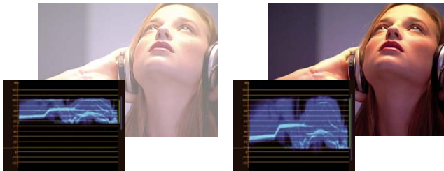
Correcting exposure: Overexposed image with the waveform in the upper limits of the IRE scale (left) and corrected image with the waveform within 7.5 to 100 IRE (right)
