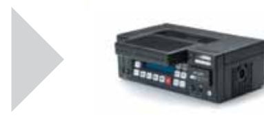
Remove the Storage Module media from Ki Pro.
